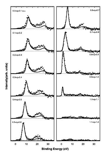
FIG. 9. The deconvoluted measured SEMD for Al at different momenta compared with the many-body cumulant expansion theory (smooth solid line). The theory was broadened with the experimental energy resolution (1.0 eV) and the momentum resolution vector (0.12, 0.1, 0.1 a.u.). A single scaling factor is used for comparison of experiment and theory.
