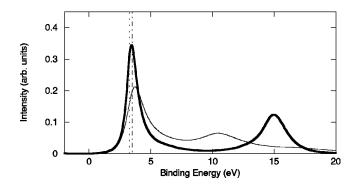
FIG. 11. Calculated spectra for Li at zero momentum using the GW approximation (thick line) and the cumulant expansion approach (thin line). The cumulant expansion spectral function peaks at slightly higher binding energy than the density calculated within the GW scheme. This is due to the larger asymmetry of the peak. The LDA energy (dash-dotted line) and the LDA energy shifted by the self-energy (short dashed) are shown for comparison.
