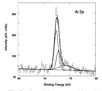
FIG. 4. The Al  $2p_{3/2,1/2}$  binding energy spectrum (relative to the Fermi level) integrated over the momentum range 0–3 a.u. The two short-dashed peaks show the  $2p_{3/2}$  and  $2p_{1/2}$  contributions of width 0.9 eV, separation of 0.4 eV, and statistical weight of 2:1. The long dashed peak is due to oxide formation and the thin line is a fit to the background produced by inelastic scattering of the electrons.
