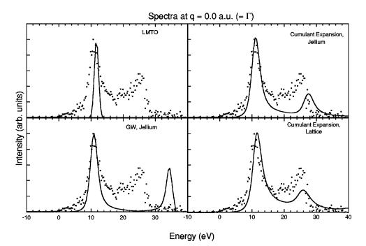
FIG. 8. The deconvoluted measured SEMD for Al at zero momentum compared with four different theories. All theories are broadened with the energy resolution. The width of the LMTO theory is equal to the experimental resolution. Further details are described in the text.
