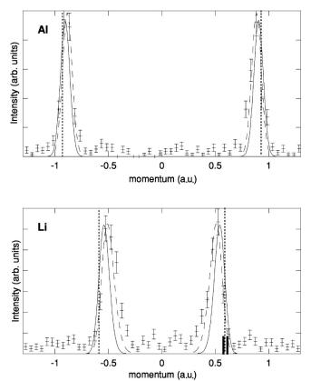
FIG. 12. The measured momentum densities for Al (top) and Li (bottom) at the Fermi level (error bars). The solid line assumes a perfect alignment. The dashed line is obtained by assuming a deviation from the ideal alignment of 0.2 a.u. Two solid bars in the right half of the lithium spectrum indicate the range of the Fermi vectors in the actual solid.
