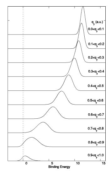
FIG. 2. Spectra at different momentum intervals as simulated with experimental momentum and energy resolution. A free electron model with  $k_F = 0.93$  a.u. was assumed  $q_x$ ,  $q_z = 0$ ,  $q_y$  as indicated.
