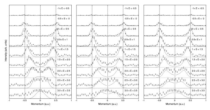
FIG. 10. Measurement of the dispersion of the lithium valence band compared to a free electron band with  $m^*=1.6m_e$  and  $k_F = 0.589$  a.u. (left panel), a cumulant expansion theory not corrected for self-energy effects (central panel) and the same calculation with an energy scale contracted by 20% (right panel).
