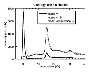
FIG. 6. The measured energy loss spectrum of 25 keV electrons scattered elastically from an Al foil over 44.3°. The intensity at 15.2 and 30.5 eV energy loss are due to single and double plasmon creation, respectively. The fitted "loss function" is used to correct the EMS data for inelastic multiple scattering as described in the text.
