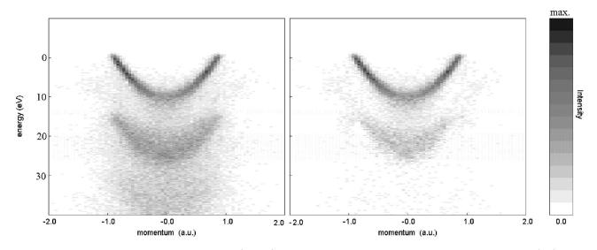
FIG. 5. The measured spectral momentum density (SEMD) in the region of the conduction band of aluminum before (left) and after (right) deconvolution for inelastic multiple scattering. The density is shown as a linear gray scale.
